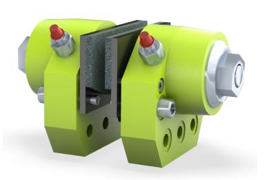
Two springs on each brake half retract the brake pads from the disc when pressure is applied. The disc spring pack must be adjusted to compensate for brake lining wear and to maintain full brake capacity. An extension of the brake piston through the adjustment nut gives an easy visual way to tell when adjustment is needed.
